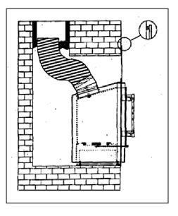
Fire stops must be installed at spaces where the chimney passes through floors and/or ceilings.
